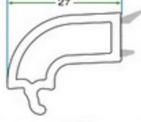
KRS 007 70'LİK ÇİFT CAM ÇİTASI KRS 006 70 DOUBLE GLASS BEAD WITH GRAY GASKET
