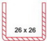
KASA DESTEK SAÇI FRAME STEEL REINFORCEMENT
