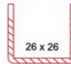
ORTA KAYIT DESTEK SAÇI MULLION STEEL REINFORCEMENT
